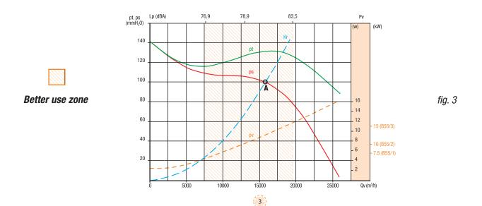
The working point is a point of equilibrium, as, in these conditions, the static pressure supplied by the fan equals the one required by the system to overcome the fluid movement resistance.
