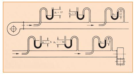
*Fig.* 1 - *Fan with outlet connected to the duct. The pressure into the duct is bigger than ambient pressure.*
